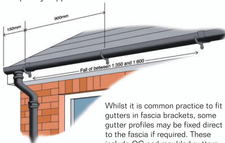
Whilst it is common practice to fit gutters in fascia brackets, some gutter profiles may be fixed direct to the fascia if required. These include OG and moulded gutters which have three pre-drilled holes per 1.8m (6') length along the top back edge.
