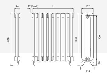
Note - When connecting bottom opposite ends 24mm must be added to 'L' dimension to allow for the reducing bushes. If connecting top/bottom same end then 12mm must be added to 'L' dimension (plus valves).
